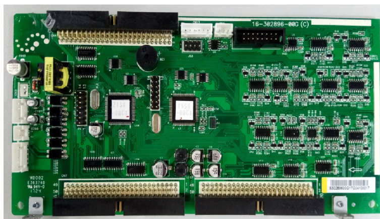
Figure 5.4.2 Arena 3/3-10K&2/2-6K Control board
